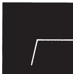
Diode in series with 51 \Omega
